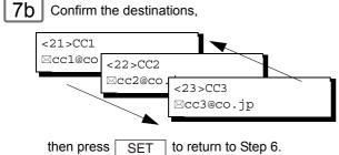
NOTE: To confirm the destinations of BCC, perform the same procedure as 7b after Step 7a.
