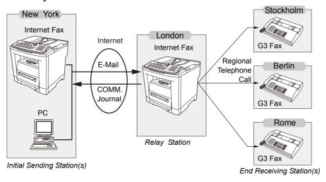
From your PC or machine, you can send documents to a Relay Station with the telephone number of the End Receiving Station(s).
