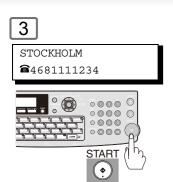
The document(s) is (are) stored into memory and your machine starts sending the document(s) to the Relay email address of the Relay Station with the telephone number for the End Receiving Station.
