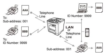
Your machine can route documents received from a G3 fax machine to email address(es) or to Internet Fax machine(s) connected to a LAN, as well as to other G3 fax machine(s) over the telephone line.
